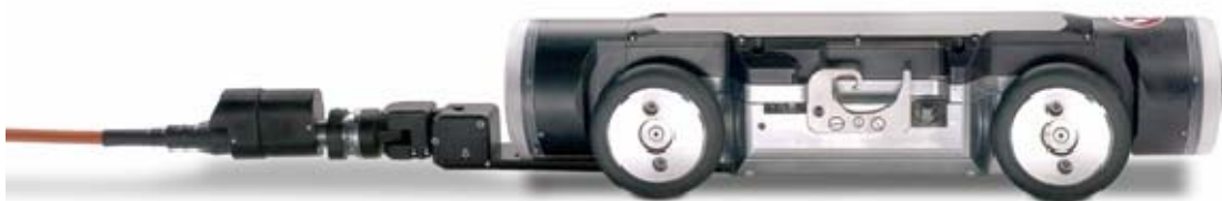
Figure 2.1 Inspection system with two symmetrically arranged scan units, each consisting of a digital photo camera and flashlighting
